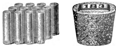
FIG. 27. — Cream sample tubes and cork stopper with numbered metal tag.
